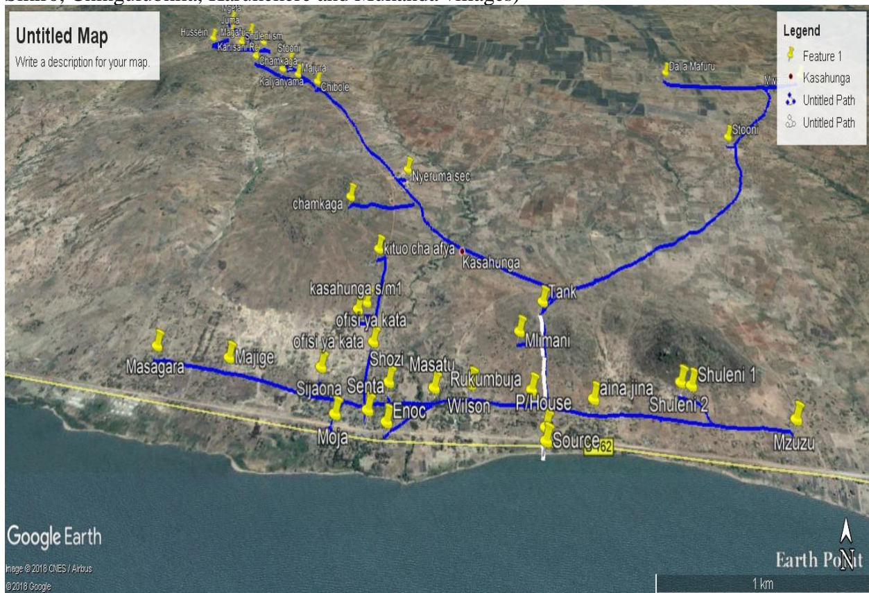
Figure 13: Proposed rehabilitation of water sources and pump house at Kasahunga, Neruma ward to pump water from Lake Victoria for up-country villages (Haruzale, Kemkombyo/Neruma, Chamakapo, Nyamitwebili and Namibu villages)
