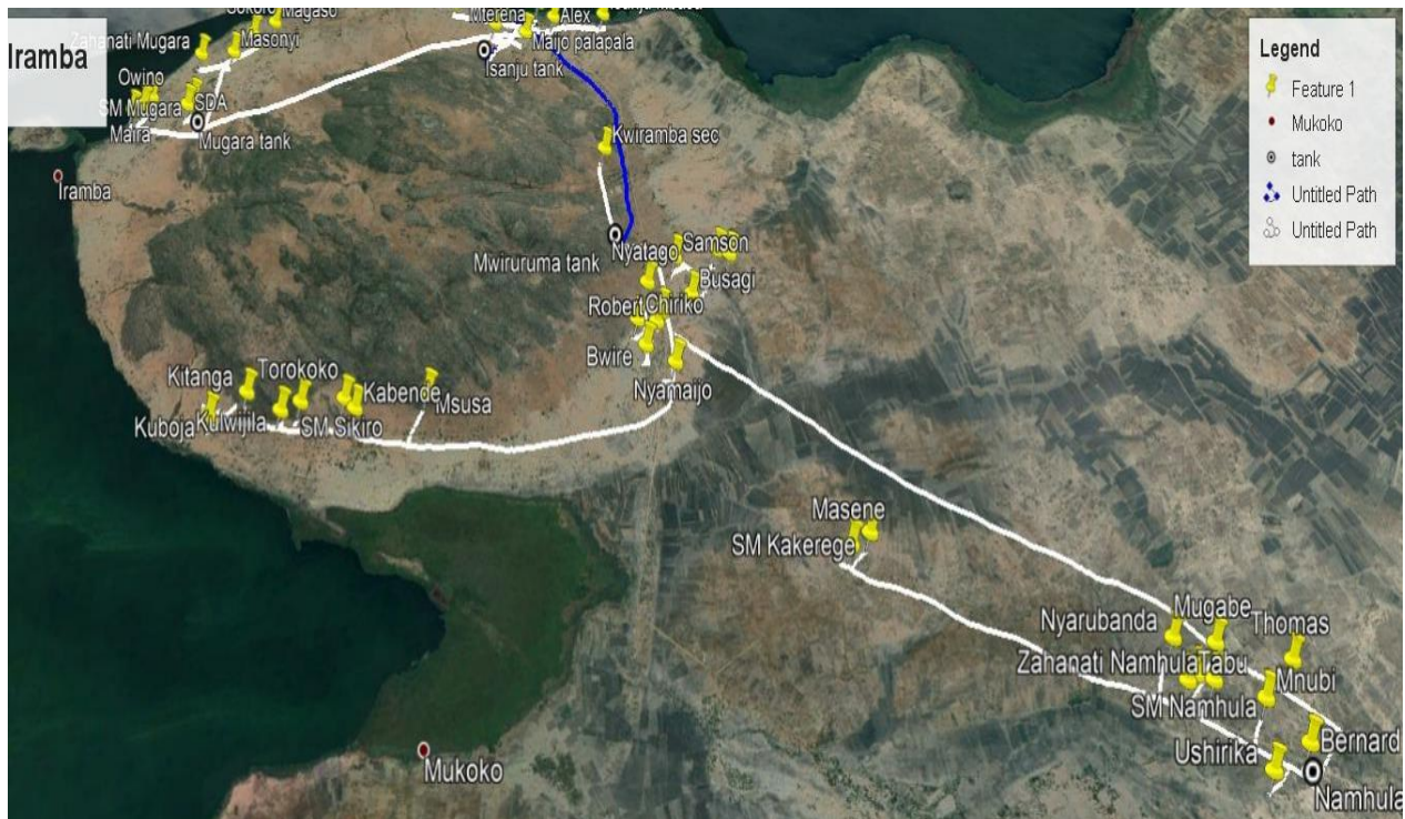
Figure 12: Proposed rehabilitation of water sources and pump house at Isanju, Iramba ward to pump water from Lake Victoria for up-country villages (Namhura, Mwiruruma, Mumaguma, Sikiro, Chingulubhila, Karukekere and Mukanda villages)
